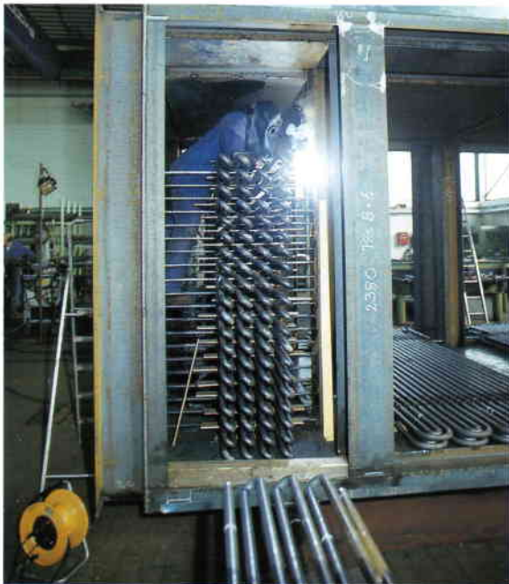
Exhaust gas boiler TT – AG 3.7 Plain tube type Evaporation 3700 kg/h Working pressure 9.0 bar
