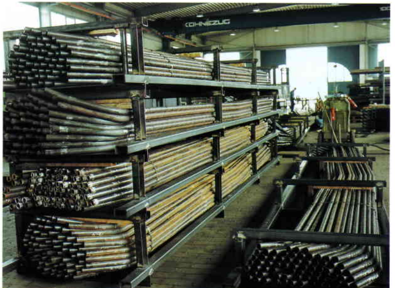
Prefabricated main bank tubes packed in crates for sea freight transport to the ship in the Arabian Gulf
