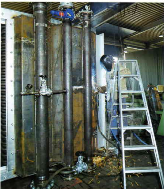
Exhaust gas boiler TT – AG 3.7 Plain tube type Evaporation 3700 kg/h Working pressure 9.0 bar
