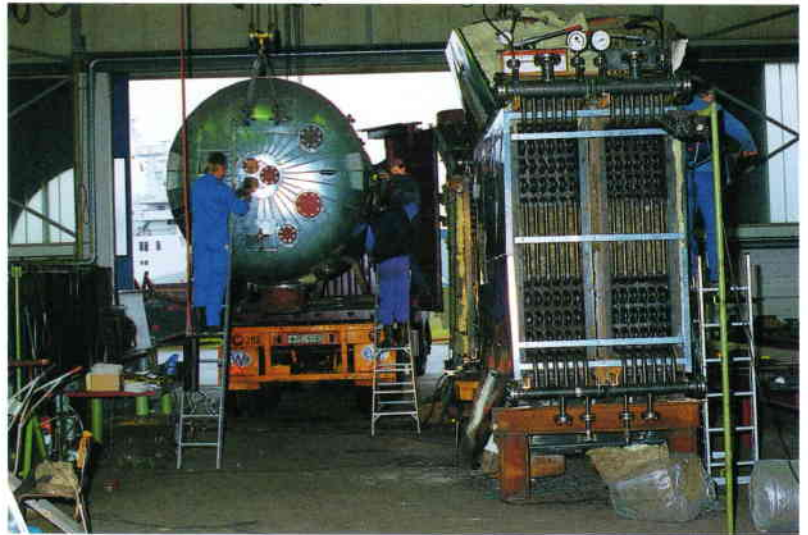
Right side: Exhaust gas boiler, double stack, finned tubes, for passenger liner.
